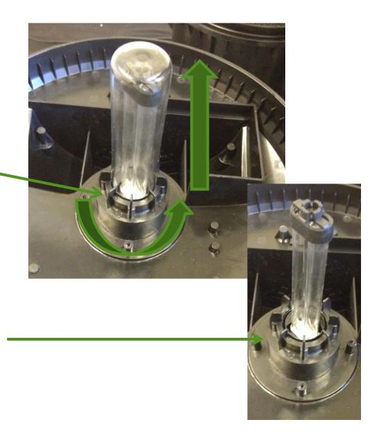
Now you are able to take out the UV bulb which is held in by pins; this will easily remove to be changed.
